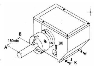
between A and B. To correct any possible difference, loosen the screw (K) clamping the headstock on the bed and adjust the headstock. Repeat this procedure until all the measurements are the same.
